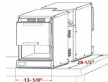
Uses only 13 5/8" (346 mm) of space (width) on a 28 ½" (724 mm) deep shelf
